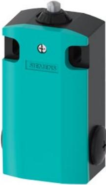
Position switch 3SE5162 Metal enclosure XL, 56 mm wide Plain plunger made of stainless steel Device connection 3 x (M20 x 1.5) 2 x (1 NO/1 NC) Quick action contacts IP66/IP67
