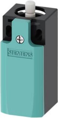
Position switch with increased corrosion protection Metal enclosure according to EN 50047, 31 mm Device connection 1 x (M20 x 1.5) 1 NO/2 NC slow-action contacts with plunger
