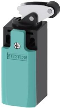
Position switch Metal enclosure according to EN 50047, 31 mm Device connection 1 x (M20 x 1.5) 1 NO/2 NC slow-action contacts Angular roller lever with plastic roller 13 mm
