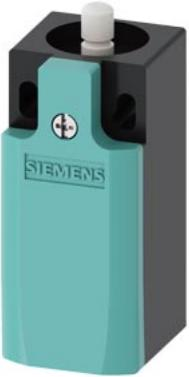
Position switch Plastic enclosure according to EN 50047, 31 mm Device connection 1 x (M20 x 1.5) 1 NO/2 NC slow-action contacts Rounded plunger, Form B with Teflon plunger functional at -40 °C Shock and vibration test according to EN 61373, Category 1B
