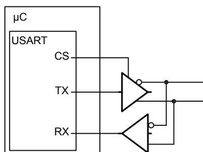
**Figure 18.10. USART Half Duplex Communication with External Driver**
