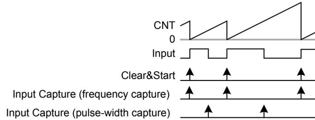
**Figure 20.13. TIMER/WTIMER Period and/or Pulse width Capture**
