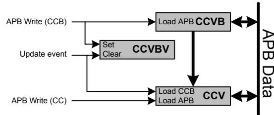
**Figure 20.16. TIMER/WTIMER Output Compare/PWM Buffer Functionality Detail**
