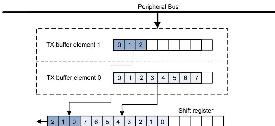
Figure 18.12. USART Transmission of Large Frames, MSBF
