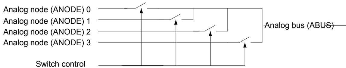
**Figure 33.1. Analog Bus (ABUS)**
