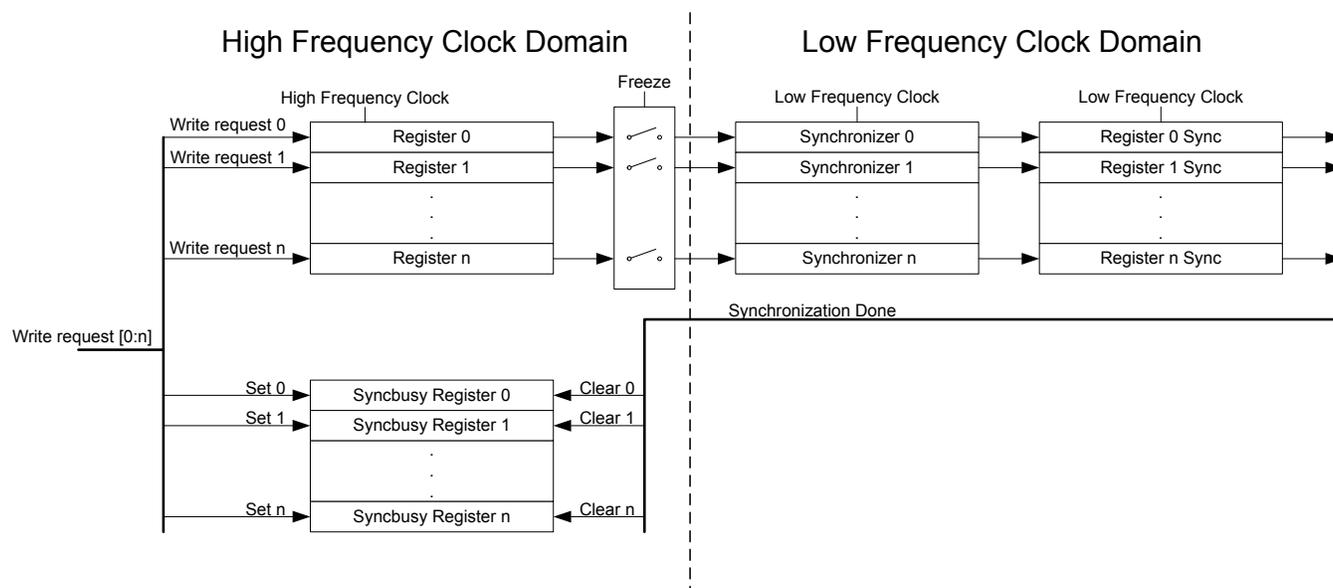
**Figure 4.12. Write Operation to Low Energy Peripherals**
