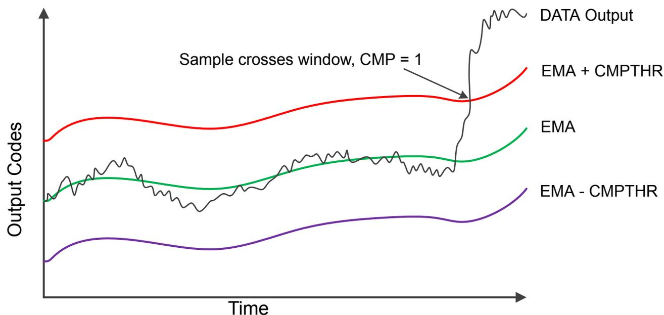
Figure 34.10. Wake on Threshold With Relative EMA
