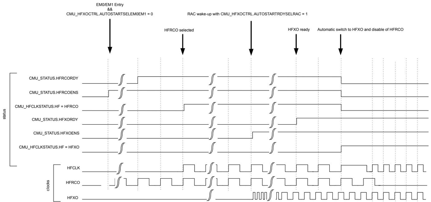
**Figure 11.10. CMU Automatic HFXO startup/selection while HFRCO started/selected**
