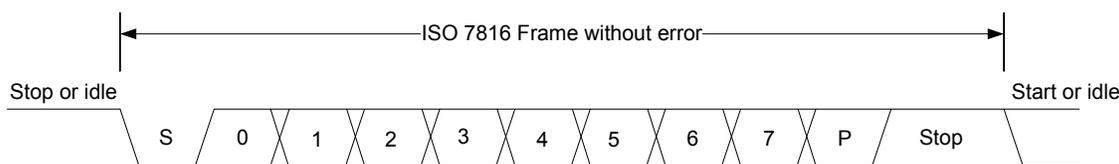
**Figure 18.14. USART ISO 7816 Data Frame Without Error**
