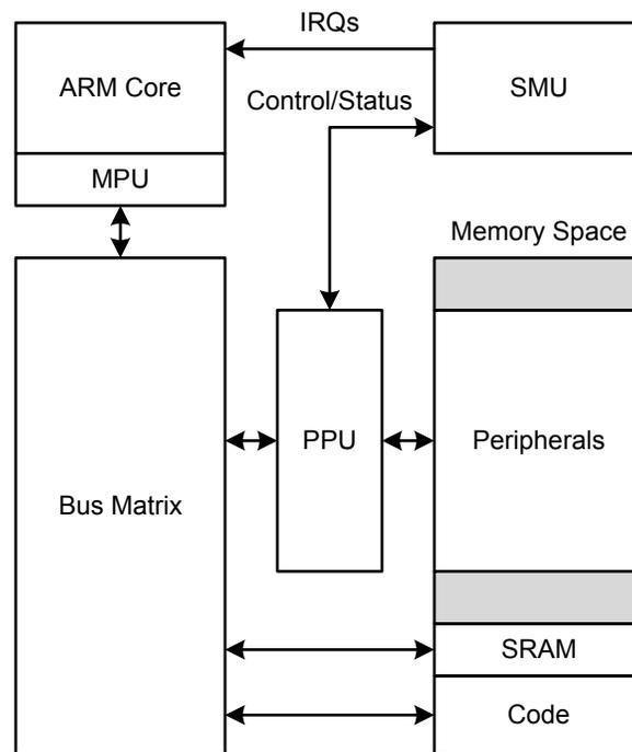
**Figure 12.1. Bus-Level Security System View**
