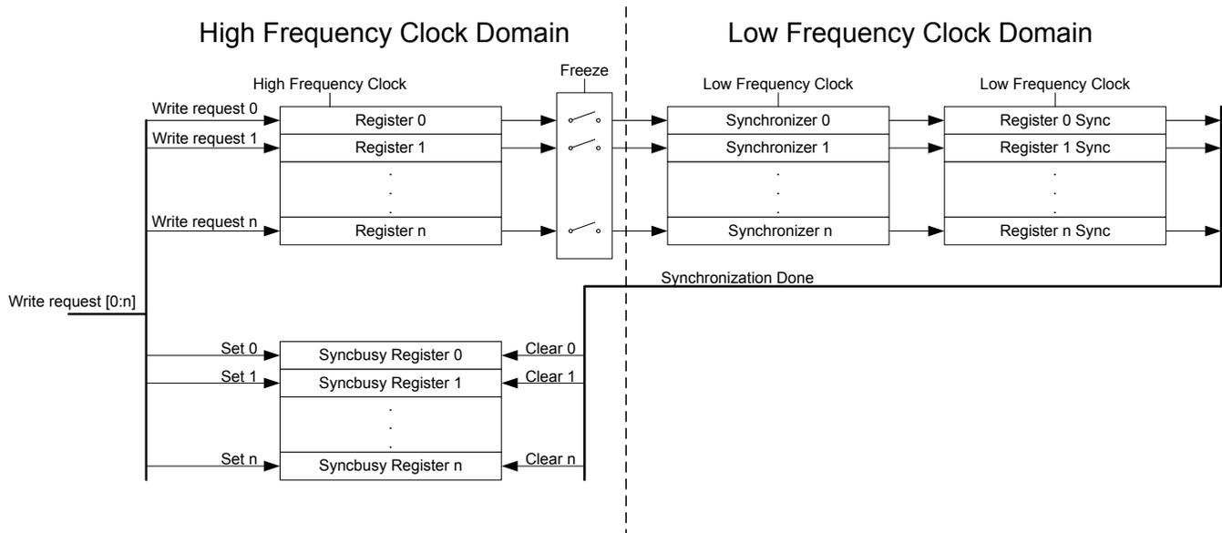
Figure 4.11. Write Operation to Low Energy Peripherals
