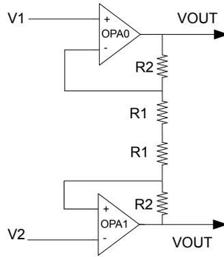
Figure 24.11. Instrumentation Amplifier Overview
