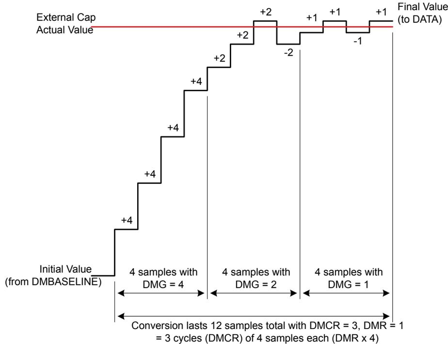
**Figure 34.2. Delta Modulation Conversion With Gain Reduction (DMCFG\_DMGRDIS = 0)**
