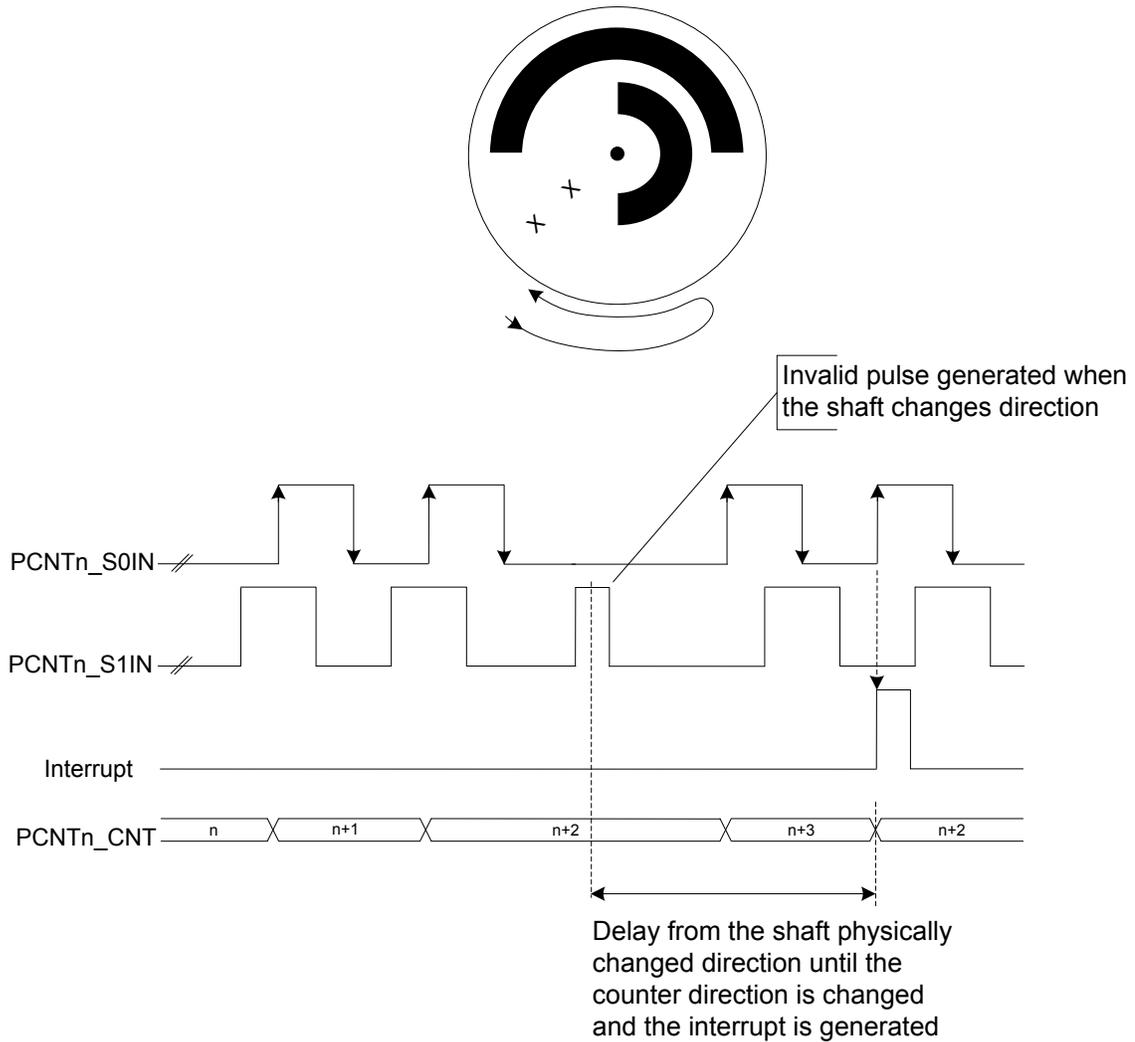
**Figure 16.13. PCNT Direction Change Interrupt (DIRCNG) Generation**
