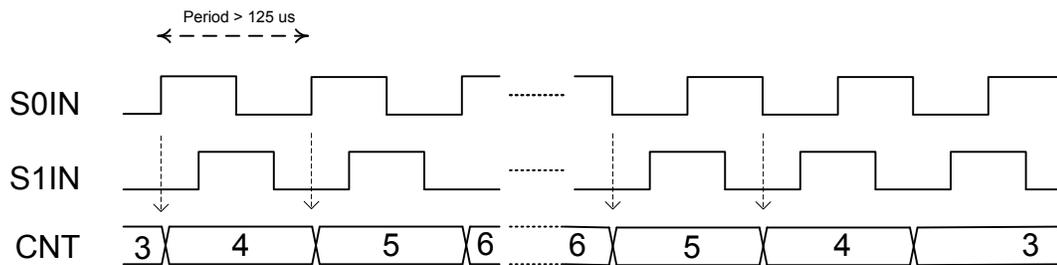
**Figure 16.4. PCNT Oversampling Quadrature Decoder 1X Mode**
