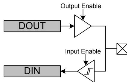
**Figure 32.3. Push-Pull Configuration**
