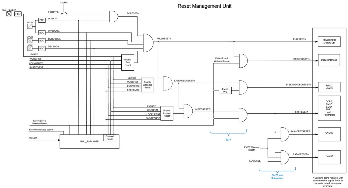
Figure 9.1. RMU Reset Input Sources and Connections
