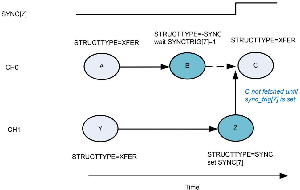
**Figure 8.8. Simple Intra-channel Synchronization Example**
