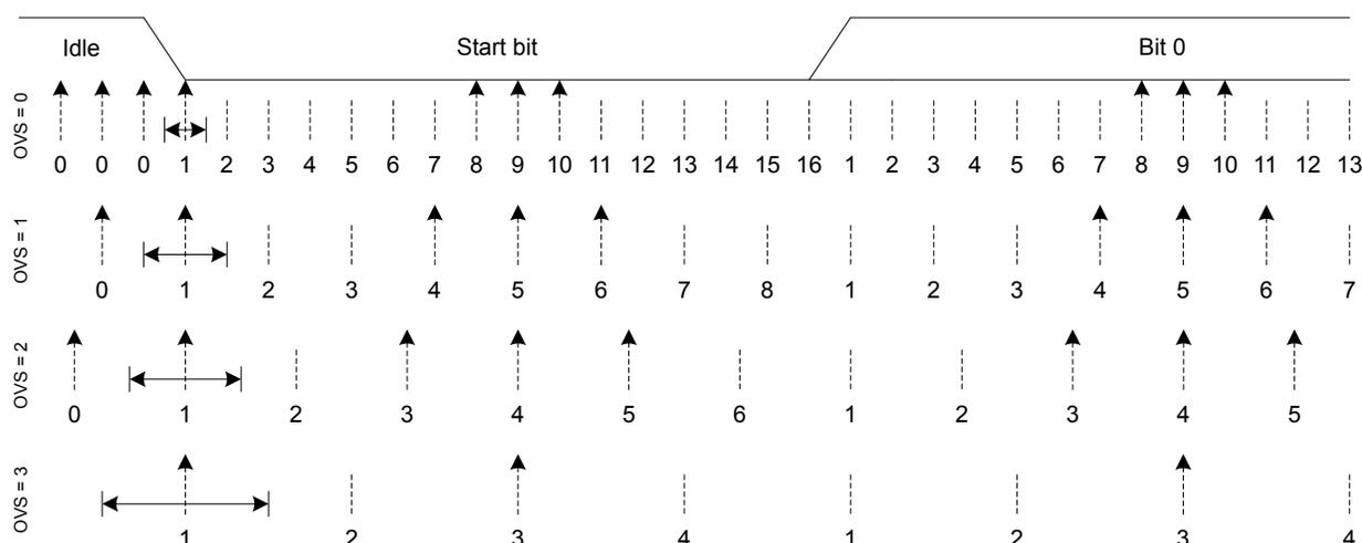
**Figure 18.7. USART Sampling of Start and Data Bits**
