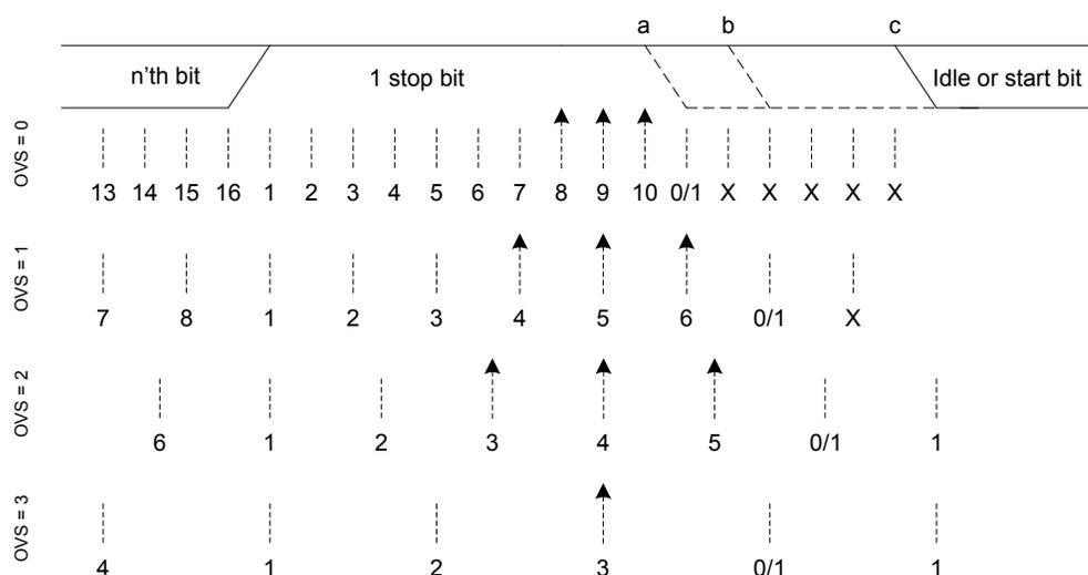
**Figure 18.8. USART Sampling of Stop Bits when Number of Stop Bits are 1 or More**
