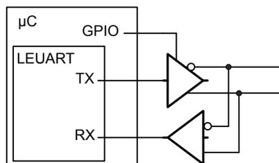
**Figure 19.10. LEUART Half Duplex Communication with External Driver**
