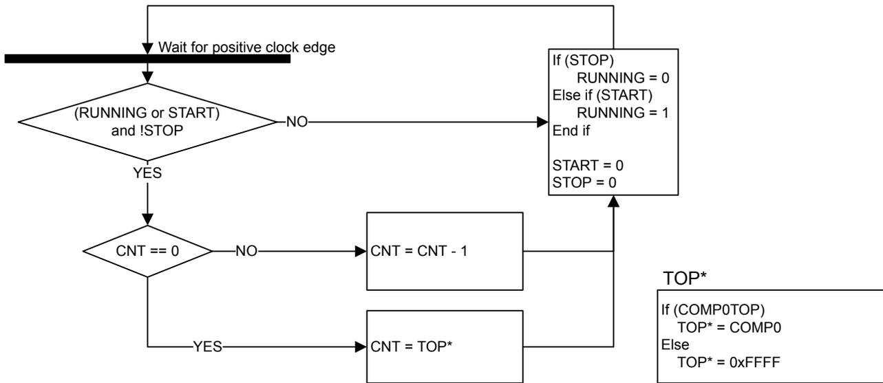
**Figure 21.2. LETIMER State Machine for Free-running Mode**
