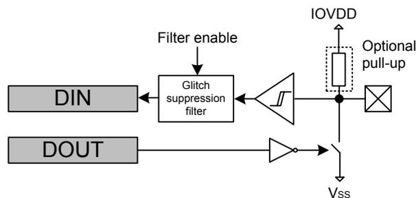
**Figure 32.4. Open-drain**
