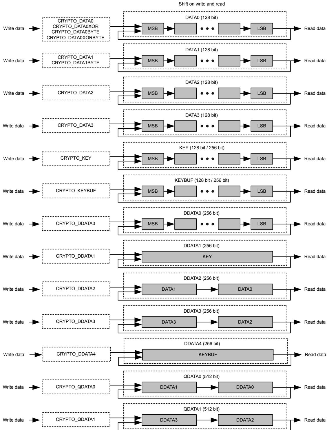
**Figure 31.2. CRYPTO Data and Key Register Operation**
