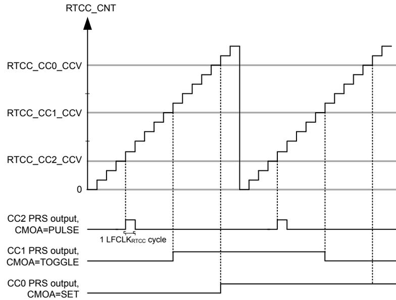
**Figure 13.3. RTCC Compare match and PRS output illustration**
