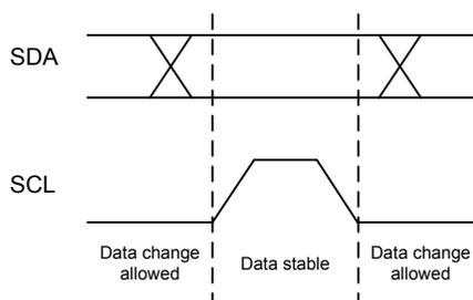
**Figure 17.5. I<sup>2</sup>C Bit Transfer on I<sup>2</sup>C-Bus**
