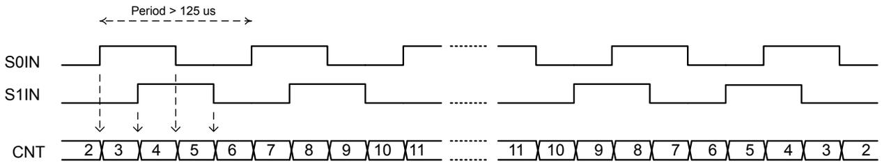
Figure 16.6. PCNT Oversampling Quadrature Decoder 4X Mode
