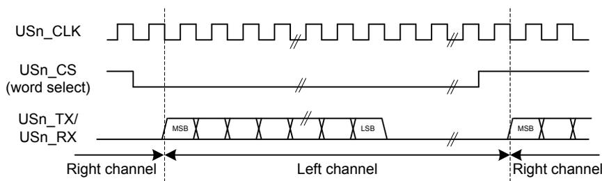
**Figure 18.21. USART Standard I2S Waveform (Reduced Accuracy)**
