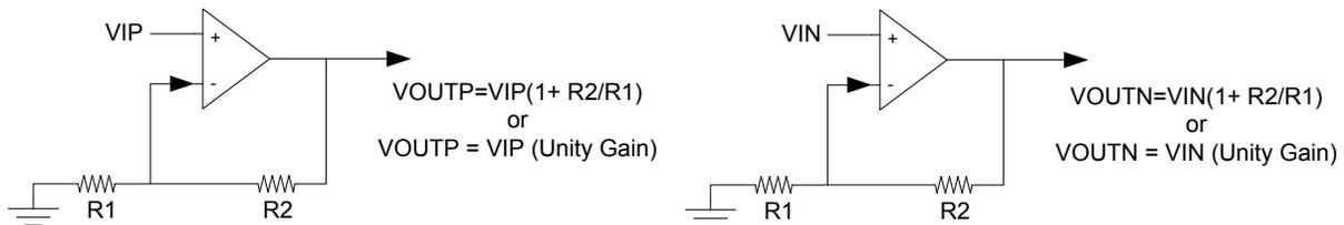
Figure 24.12. Dual Buffer ADC Driver Overview
