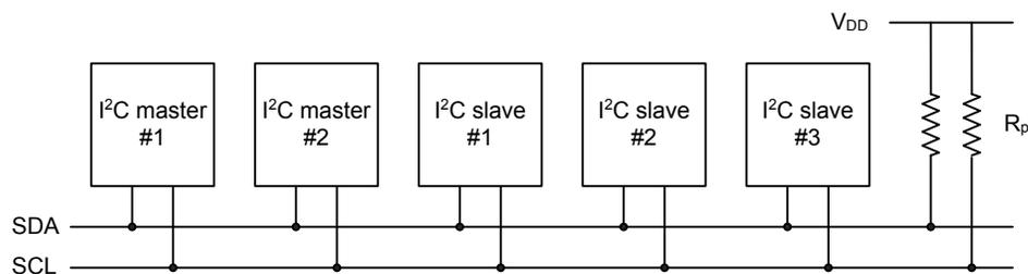
**Figure 17.2. I<sup>2</sup>C-Bus Example**
