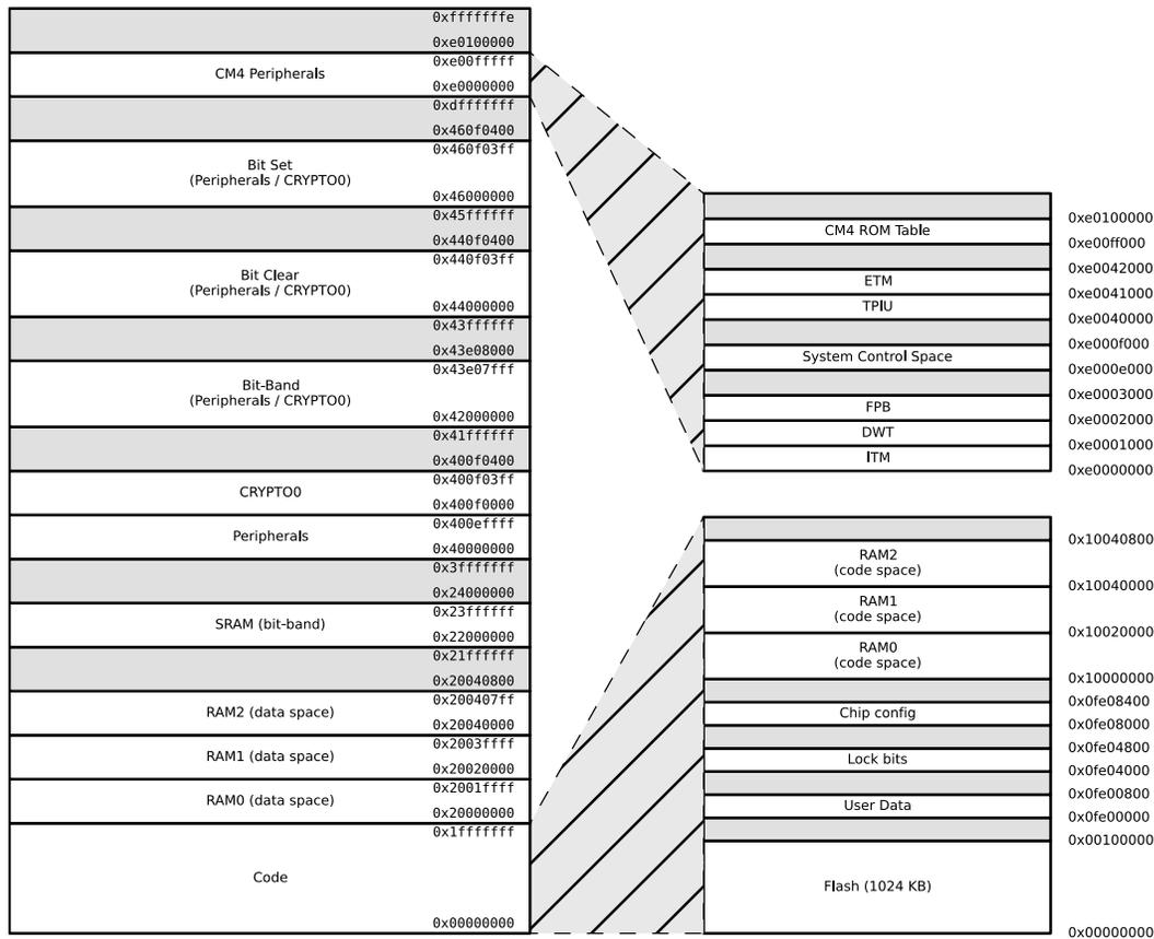
**Figure 4.2. System Address Space With Core and Code Space Listing**
