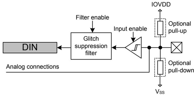
**Figure 32.2. Tristated Output With Optional Pull-up or Pull-down**
