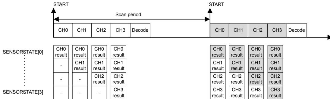
**Figure 28.10. Sensor Scan and Decode Sequence**
