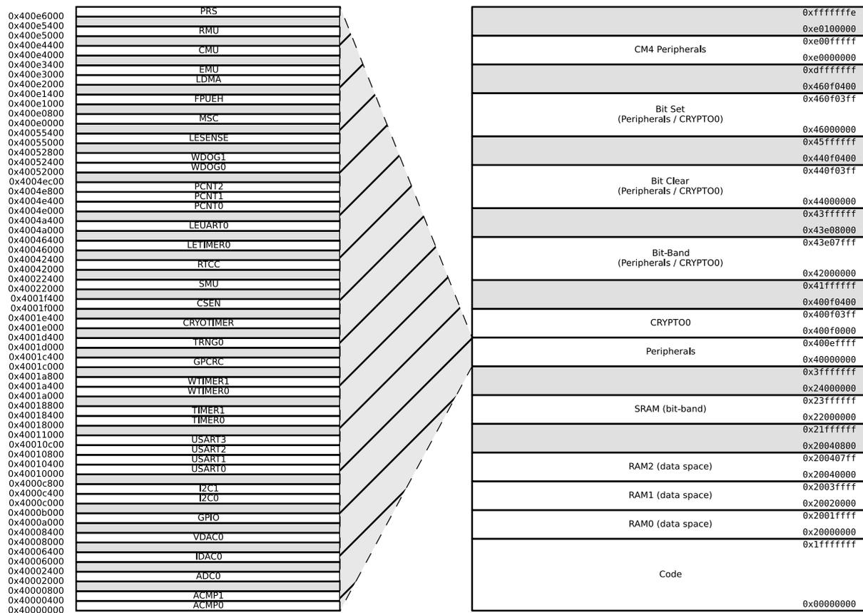
Figure 4.3. System Address Space With Peripheral Listing
