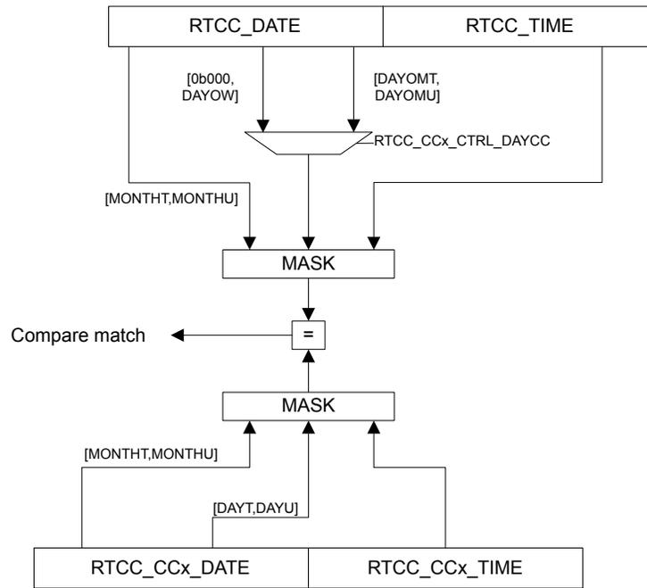
Figure 13.5. RTCC Compare in calendar mode, COMPBASE = CNT
