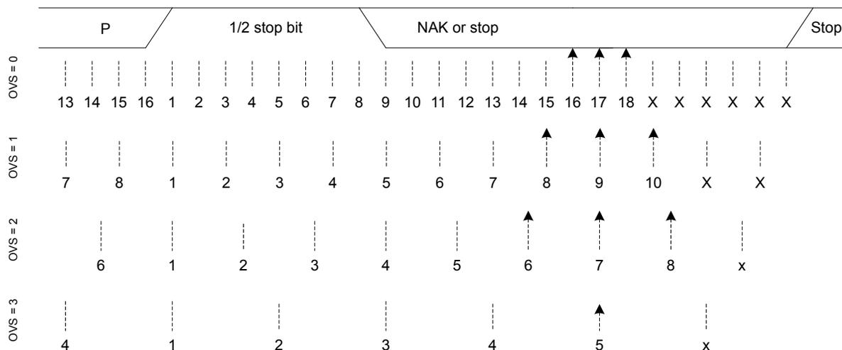
**Figure 18.16. USART SmartCard Stop Bit Sampling**
