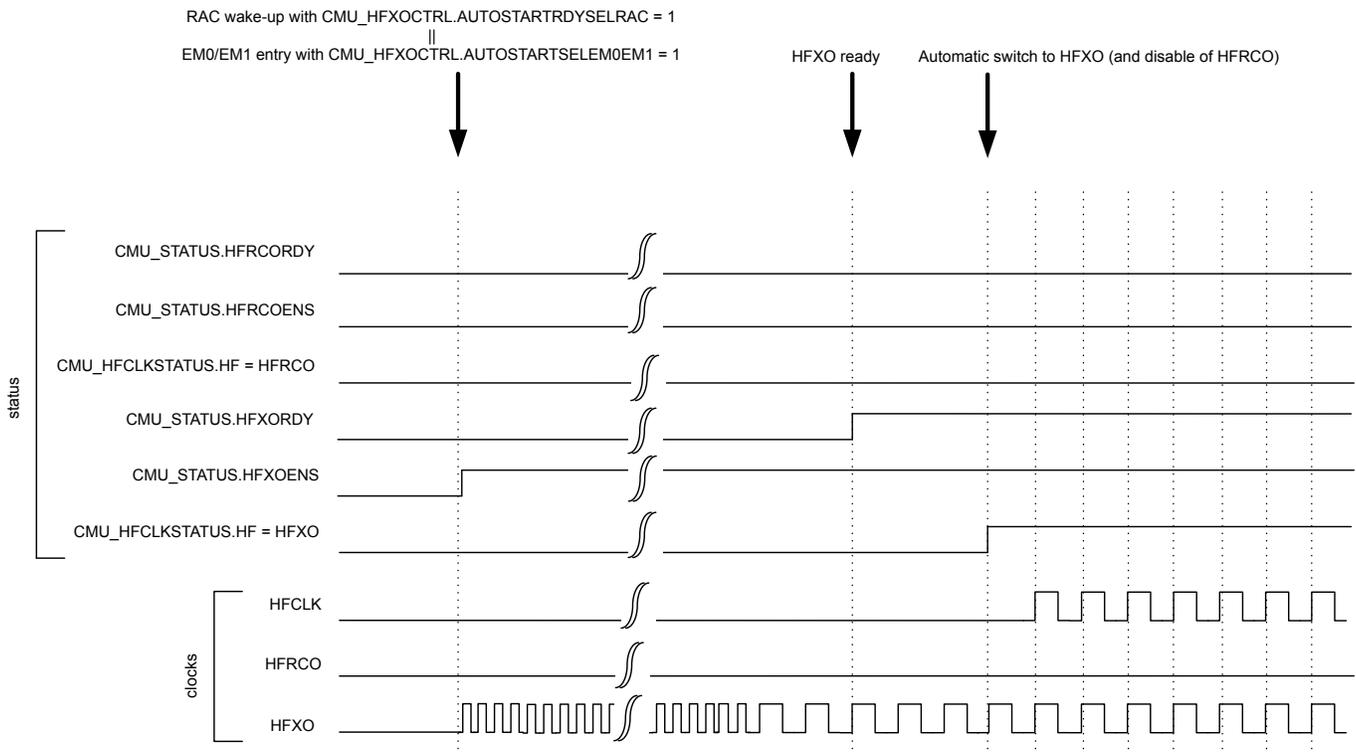
**Figure 11.8. CMU Automatic Startup and Selection of HFXO**
