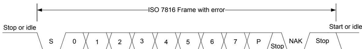
**Figure 18.15. USART ISO 7816 Data Frame With Error**
