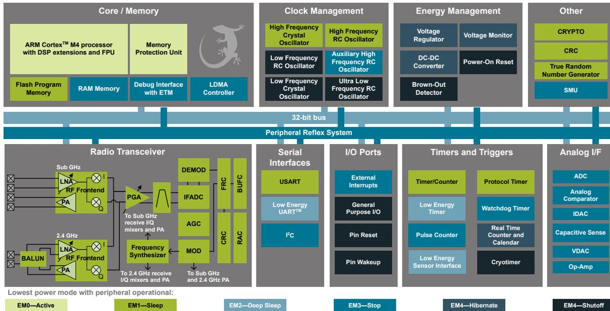
Figure 2.1. EFR32xG12 Wireless Gecko System-On-Chip Block Diagram
