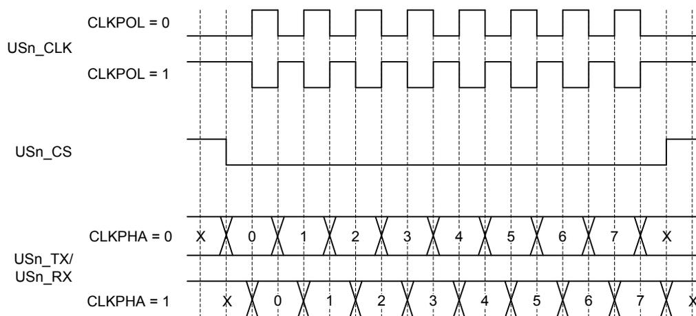
**Figure 18.19. USART SPI Timing**
