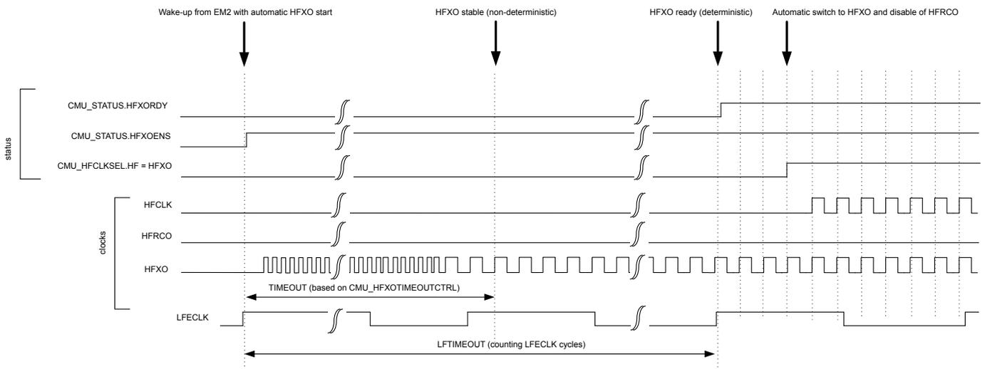
**Figure 11.3. CMU Deterministic HFXO startup using LFTIMEOUT**
