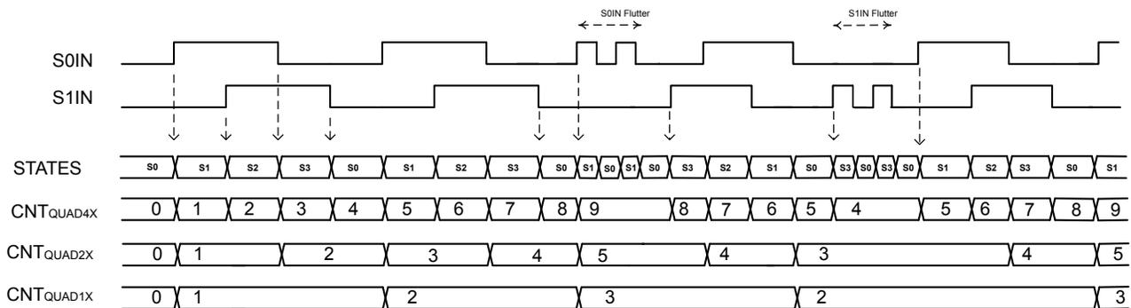
Figure 16.7. PCNT Oversampling Quadrature Decoder with Flutter Removal
