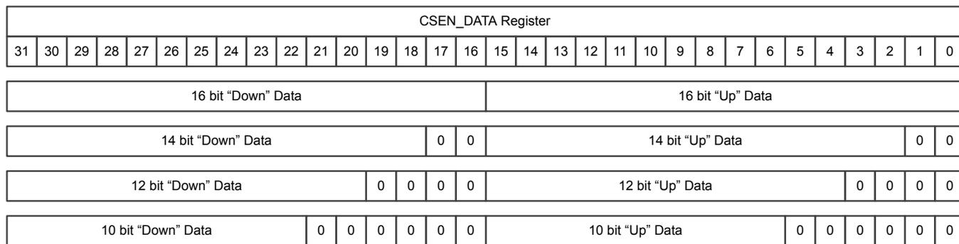
**Figure 34.8. Data Encoding for Delta Modulation With Chopping**
