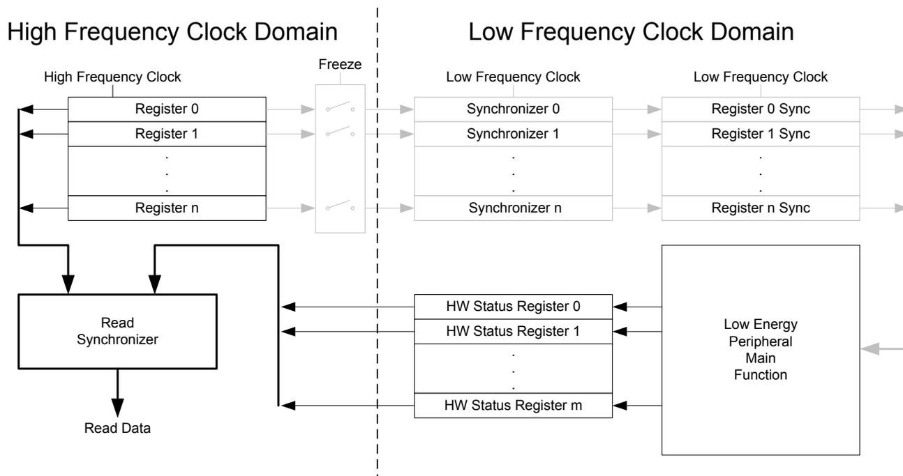
Figure 4.13. Read Operation From Low Energy Peripherals
