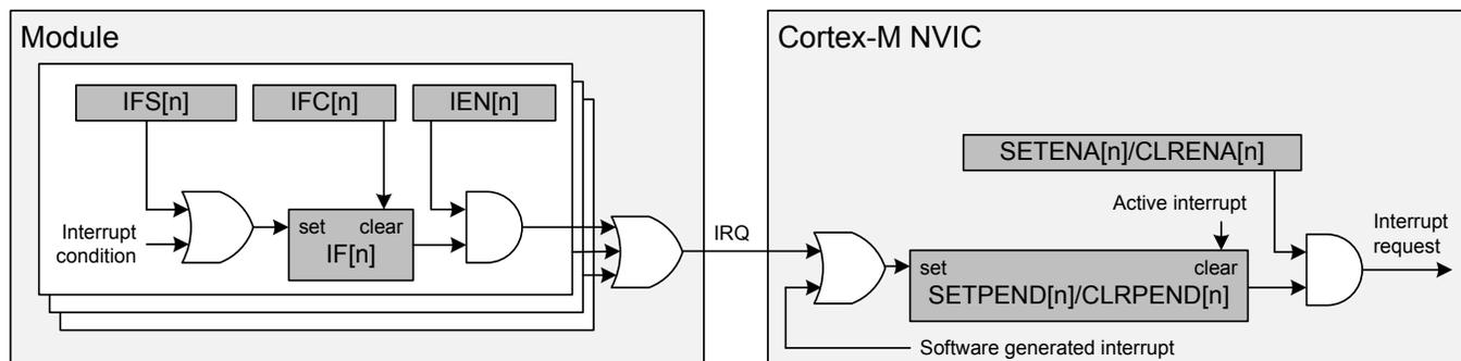
Figure 3.1. Interrupt Operation
