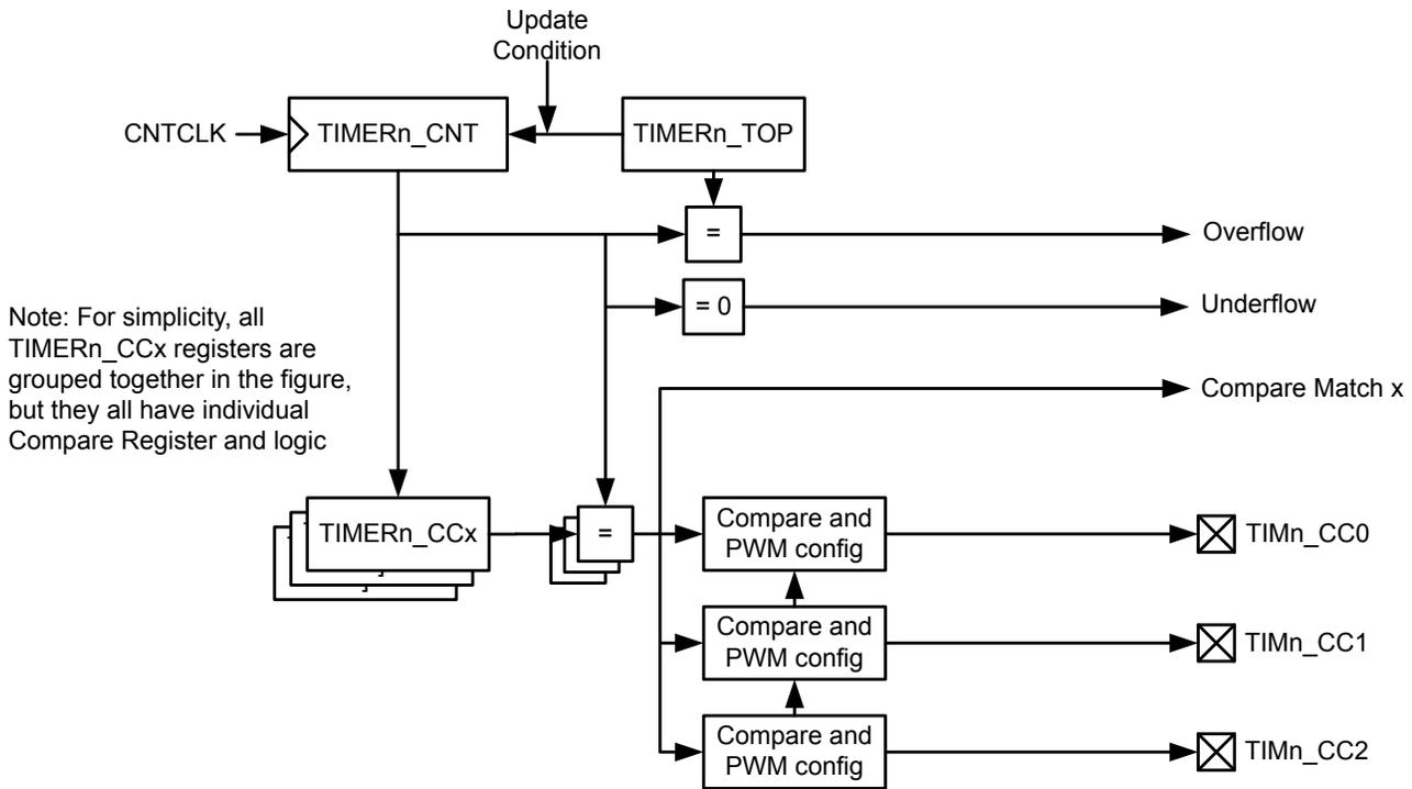
**Figure 20.14. TIMER/WTIMER Block Diagram Showing Comparison Functionality**
