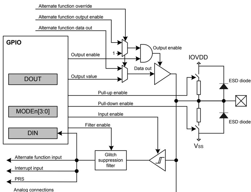
Figure 32.1. Pin Configuration
