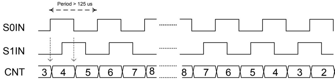
Figure 16.5. PCNT Oversampling Quadrature Decoder 2X Mode
