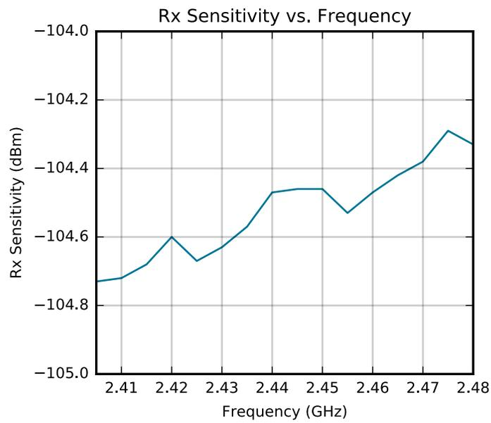
Figure 4.9. 2.4 GHz 802.15.4 RF Receiver Sensitivity
