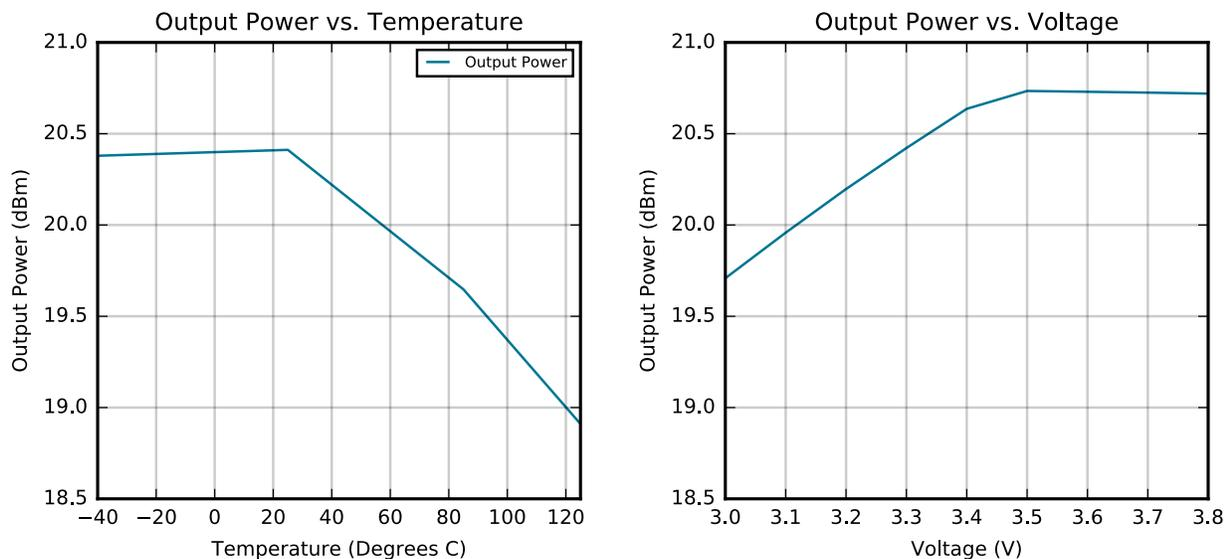
Figure 4.6. 2.4 GHz 20 dBm PA RF Transmitter Output Power
