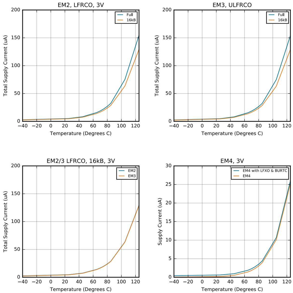
Figure 4.15. EM2, EM3, and EM4 Sleep Mode Typical Supply Current vs. Temperature
