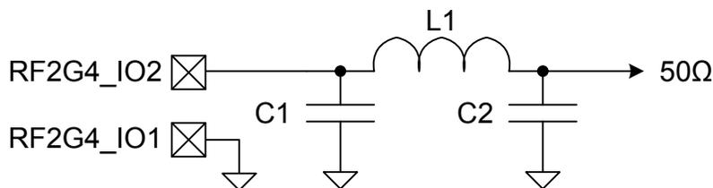
Figure 5.3. Typical 10 dBm 2.4 GHz RF impedance-matching network circuit
