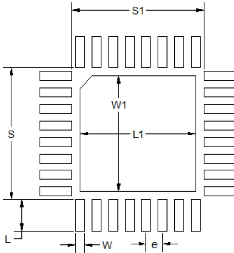
Figure 7.2. QFN32 PCB Land Pattern Drawing
