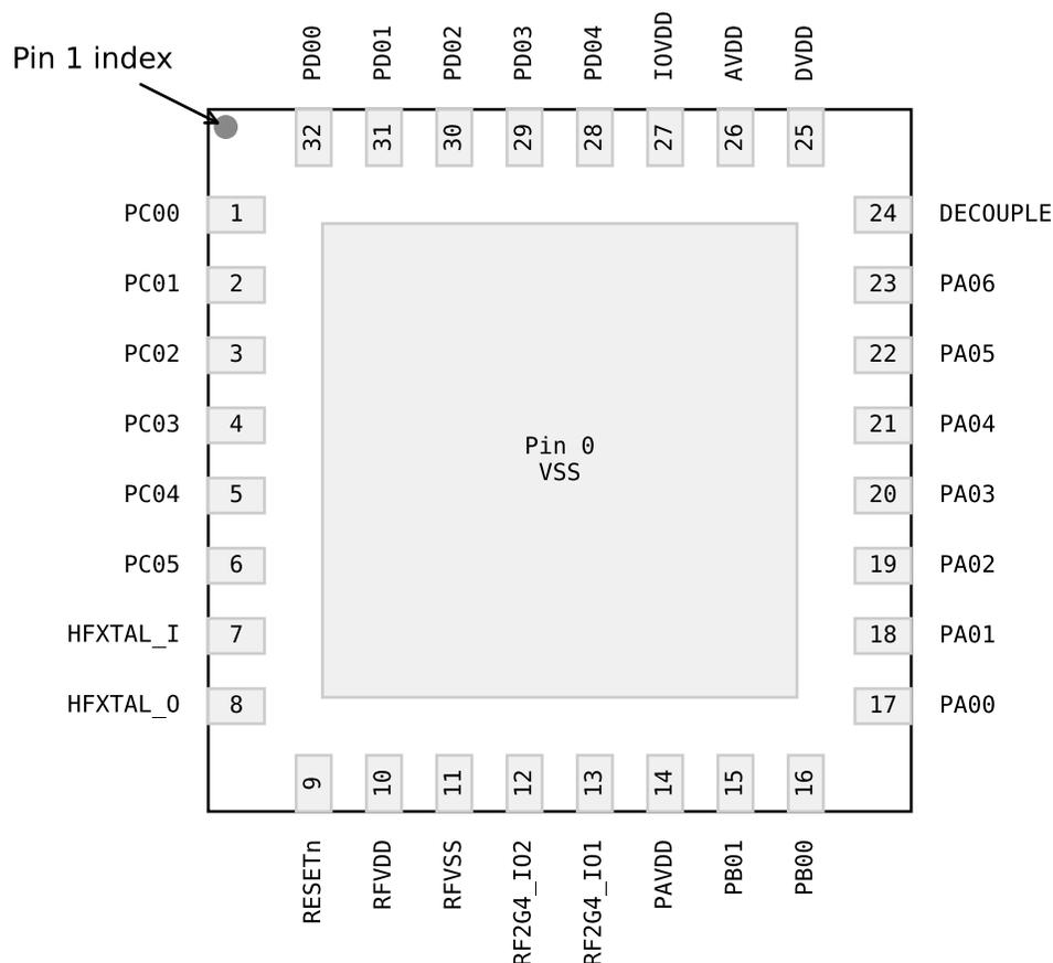
Figure 6.1. QFN32 Device Pinout
