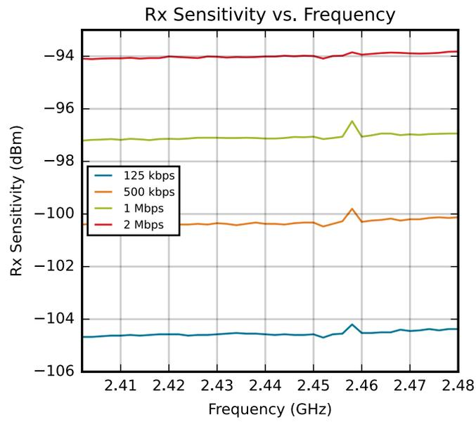
Figure 4.20. 2.4 GHz BLE RF Receiver Sensitivity
