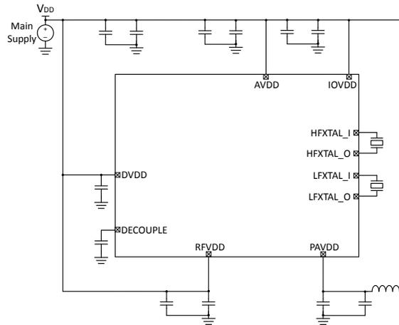
Figure 5.1. EFR32MG21 Typical Application Circuit: Direct Supply Configuration
