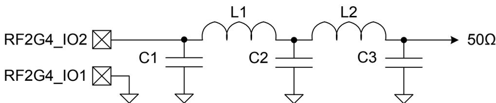
Figure 5.4. Typical 20 dBm 2.4 GHz RF impedance-matching network circuit
