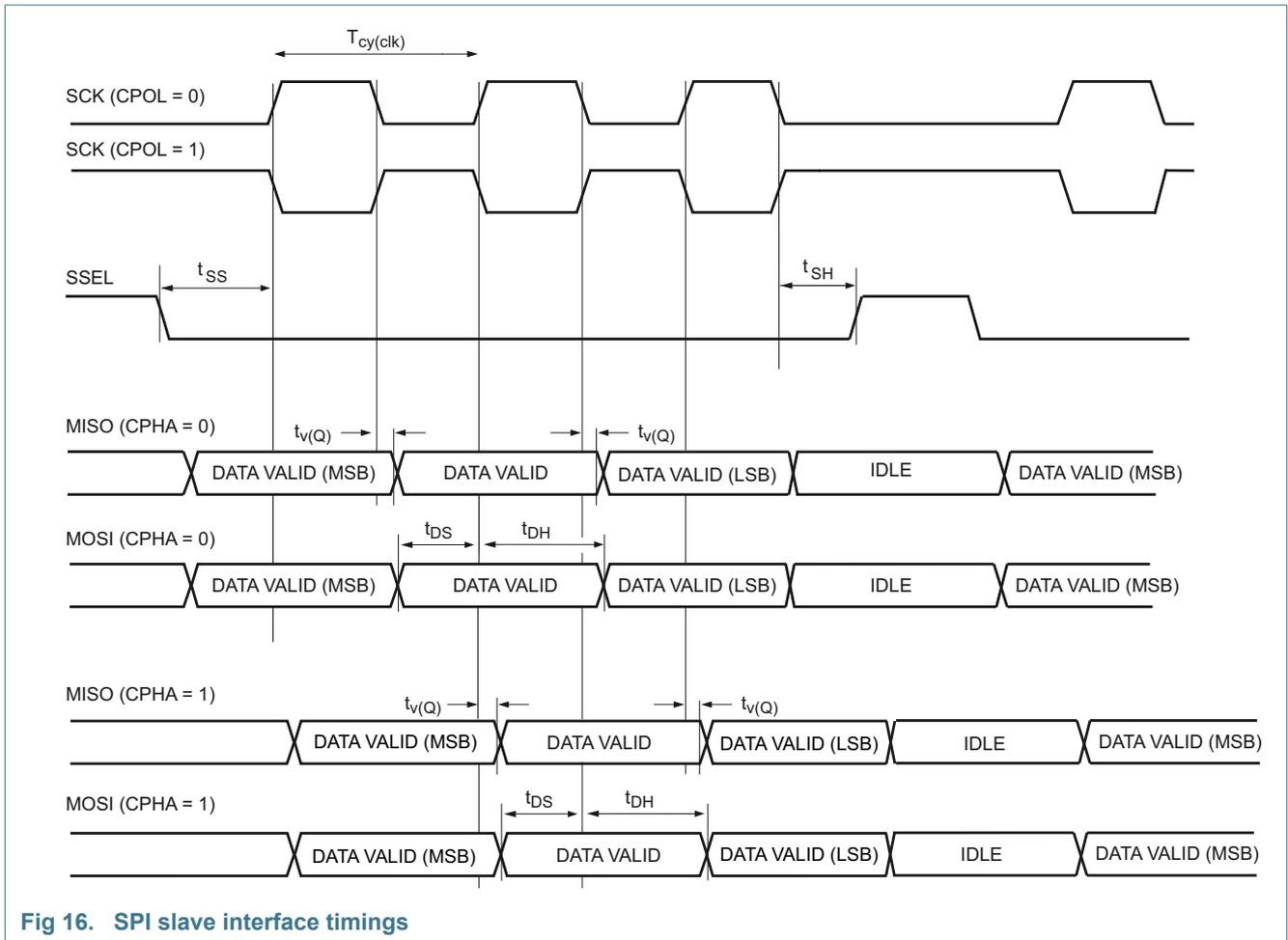
Fig 16. SPI slave interface timings
