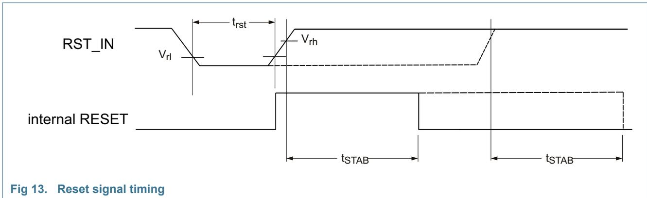
**Fig 13. Reset signal timing**
