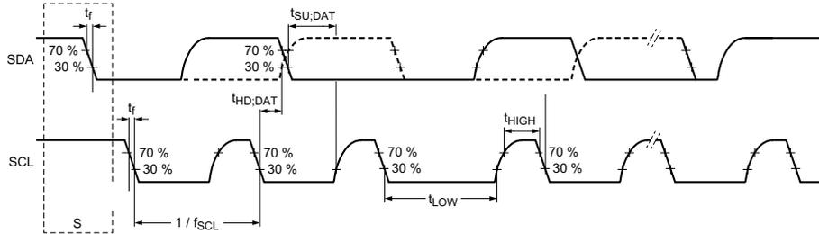
Fig 20. I<sup>2</sup>C interface timings
