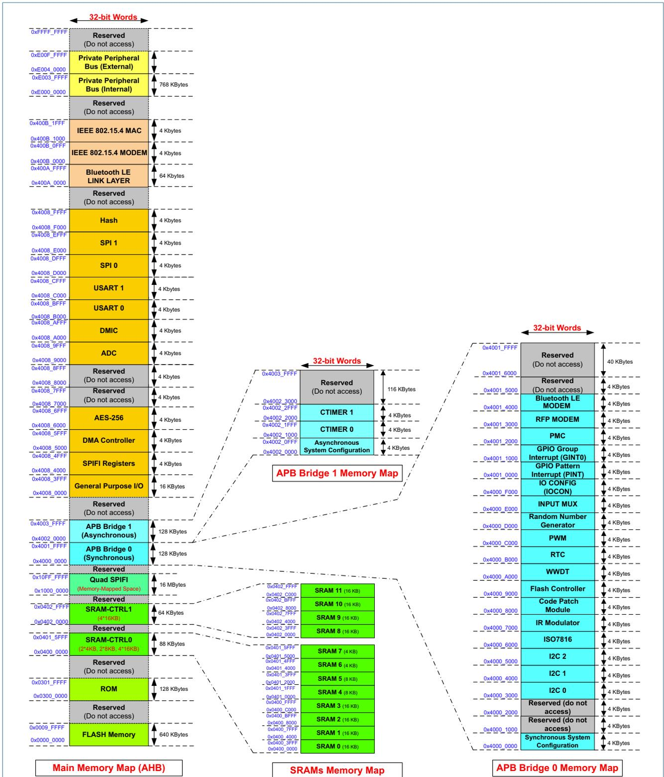
1) The private peripheral bus includes CPU peripherals such as the NVIC, SysTick, and the core control registers.
