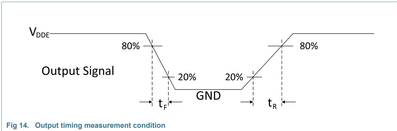
**Fig 14. Output timing measurement condition**
