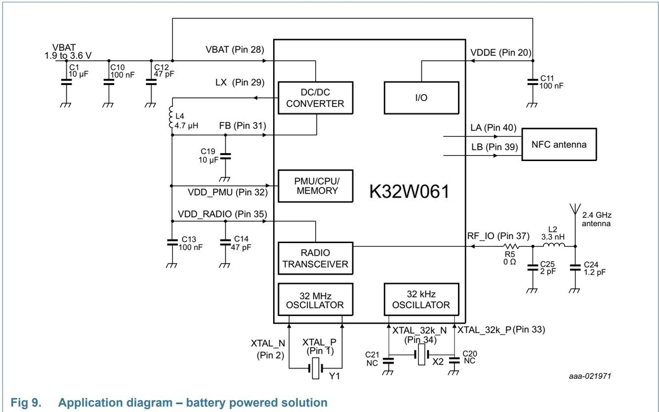
**Fig 9. Application diagram – battery powered solution**
