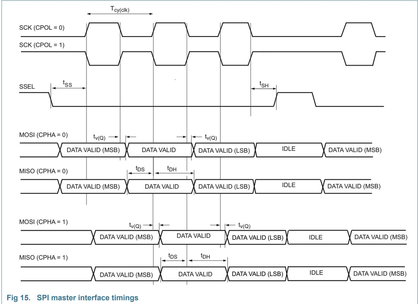
Fig 15. SPI master interface timings
