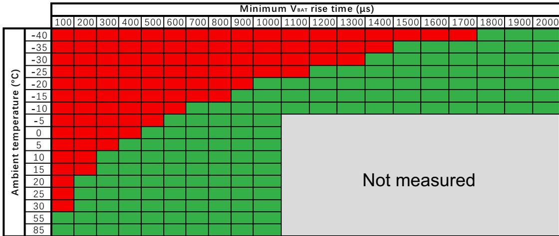
Fig 11. Minimum  $V_{BAT}$  rise time vs temperature
