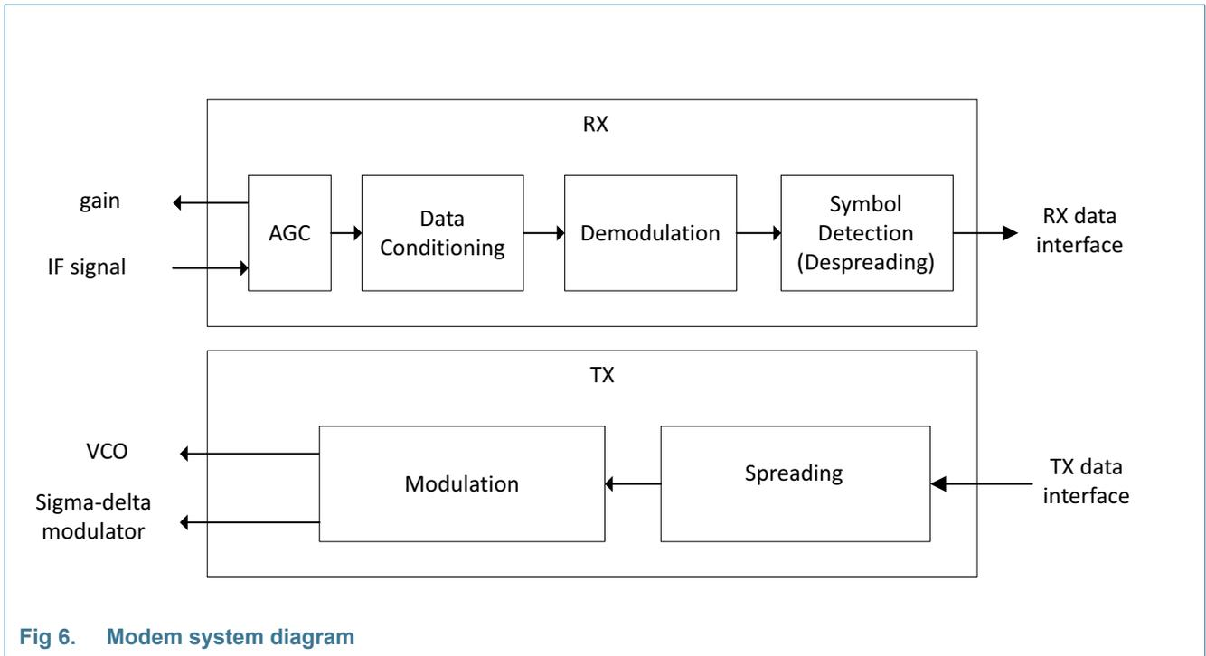
**Fig 6. Modem system diagram**
