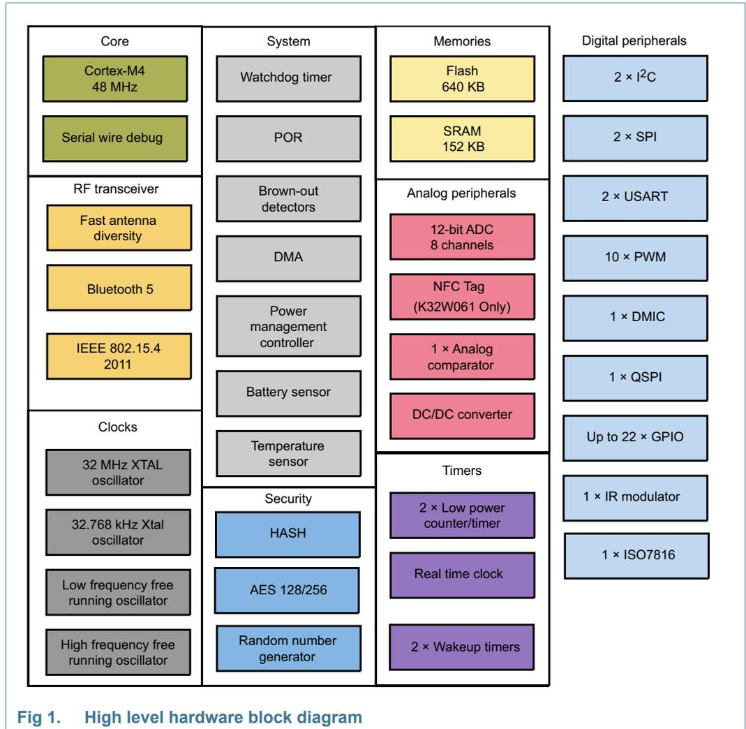
Fig 1. High level hardware block diagram
