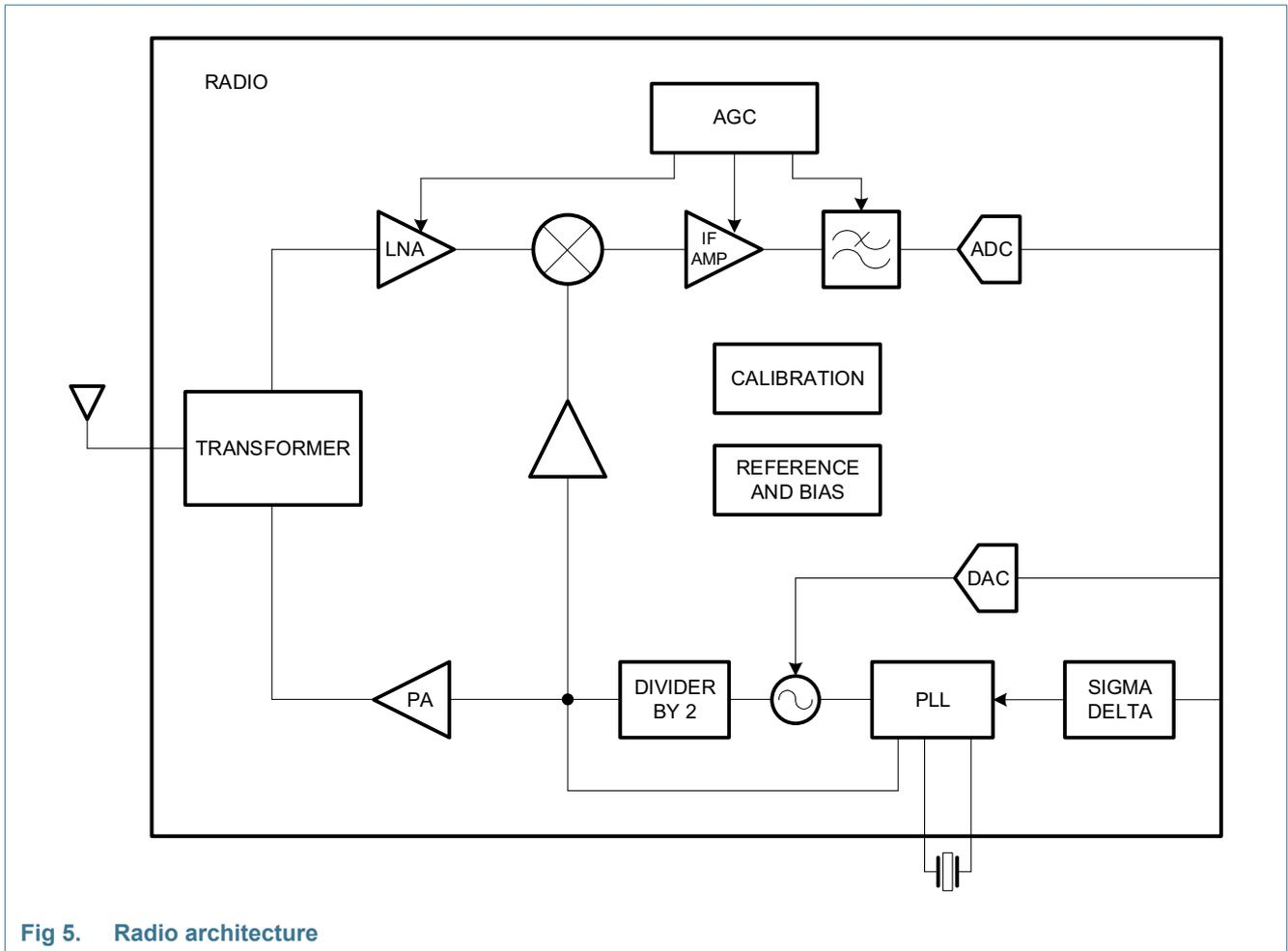
Fig 5. Radio architecture
