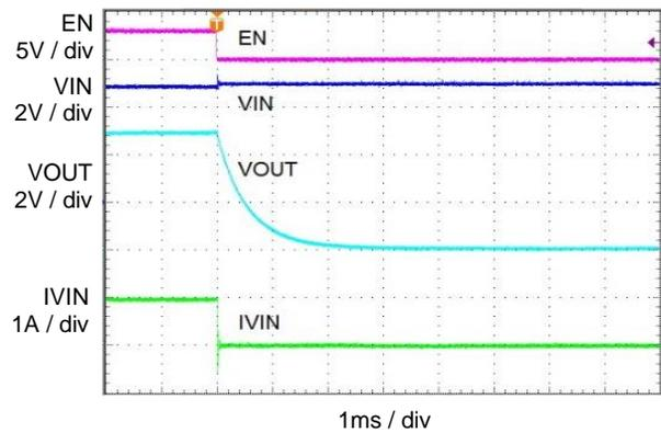
**Device Enabled into Current Limit Mode**
