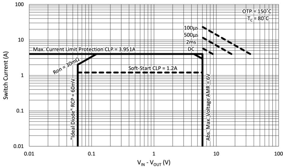
**Figure 5. Safe Operating Area (SOA) for  $T_C = 80^\circ\text{C}$**
