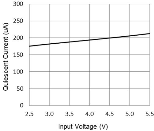
**Shutdown Supply Current vs.  $V_{IN}$**
