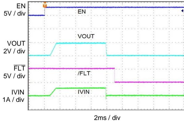
**Load Increase Trigger Current Limit**
