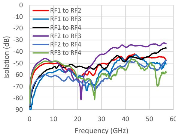
**Isolation between RF1 to RF4, RFC to RF4 On<sup>11</sup>**
