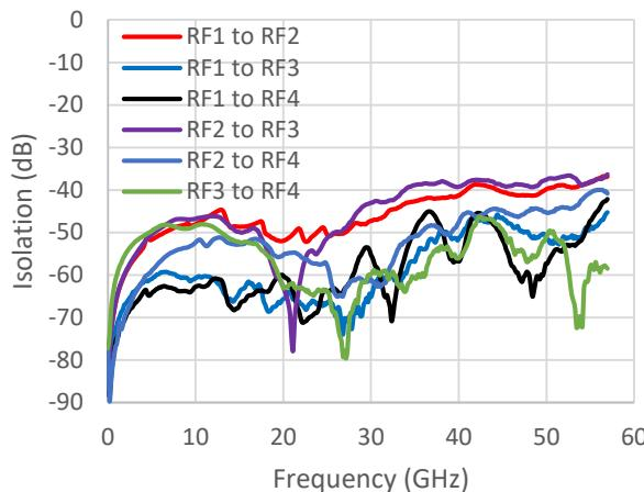
**Isolation between RF1 to RF4, RFC to RF3 On<sup>11</sup>**
