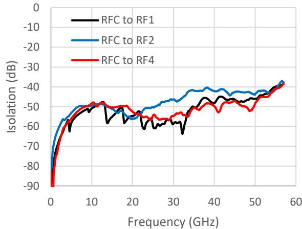
**Isolation between RF1 to RF4, RFC to RF1 On<sup>11</sup>**
