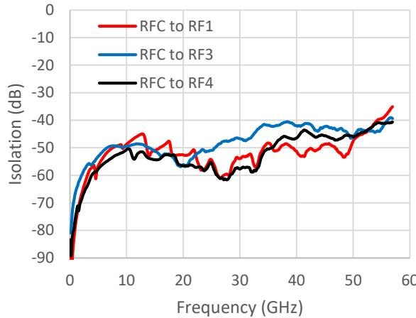
**RFC to RF1 / RF2 / RF4 Isolation, RFC to RF3 On<sup>11</sup>**
