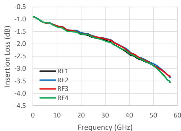
**RFC to RF1/RF4 Insertion Loss over Temperature<sup>11</sup>**
