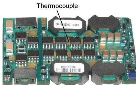
Figure 5. Location of the thermocouple for thermal testing
