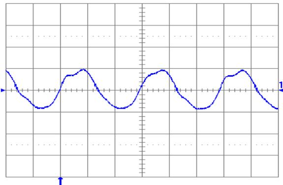
Figure 20. Output voltage ripple (20 mV/div.) at full rated load current into a resistive load with  $C_o = 10\text{ }\mu\text{F}$  tantalum + 1  $\mu\text{F}$  ceramic and  $V_{in} = 48\text{ V}$ . Time scale: 1  $\mu\text{s}$ /div.
