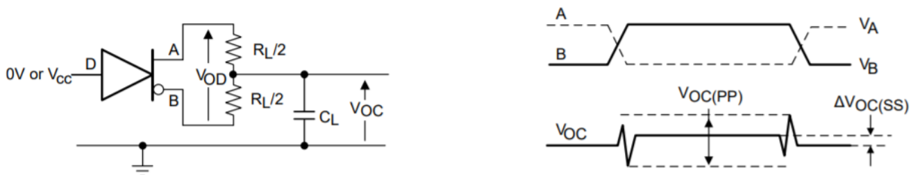
Figure 4. Driver Propagation Delay and Rise/Fall Time Measurement
